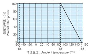
在环境温度85℃以上使用时,应按照上图负荷减轻特性曲线,减小额定功率。 For resistors operated at an ambient temperature of 85°C or above, a power rating shall be derated in accordance with the above derating curve.
