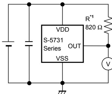
\*1. Resistor (R) is unnecessary for the pull-up resistor built-in product.
