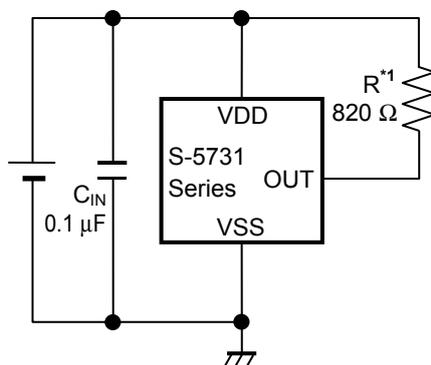
\*1. Resistor (R) is unnecessary for the pull-up resistor built-in product.
