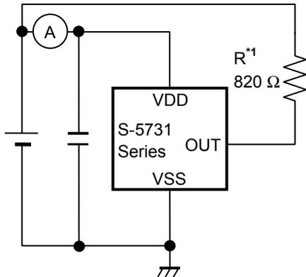
\*1. Resistor (R) is unnecessary for the pull-up resistor built-in product.
