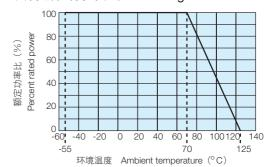
在环境温度70℃以上使用时,应按照上图负荷减轻特性曲线曲线,减小额定功率。 For resistors operated at an ambient temperature of 70°C or above, a power rating shall be derated in accordance with the above derating curve.
