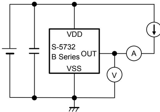
**Figure 6 Test Circuit 2**
