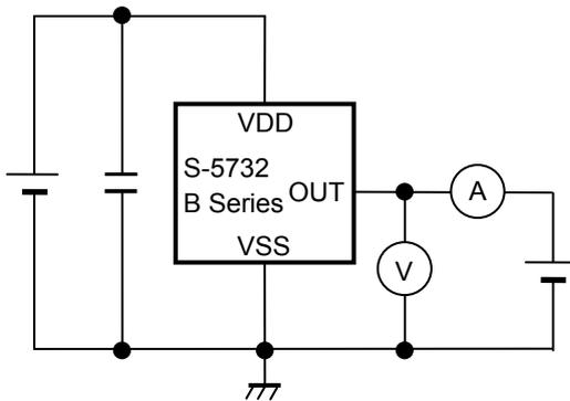
**Figure 7 Test Circuit 3**
