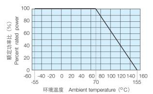
在环境温度70°C以上使用时,应按照左图负荷减轻特性曲线,减小额定功率。 For resistors operated at an ambient temperature of 70°C or above, a power rating shall be derated in accordance with the left derating curve.
