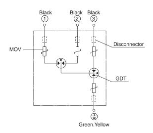
Flexible wires in black color can connect to each phase without any specific control.
