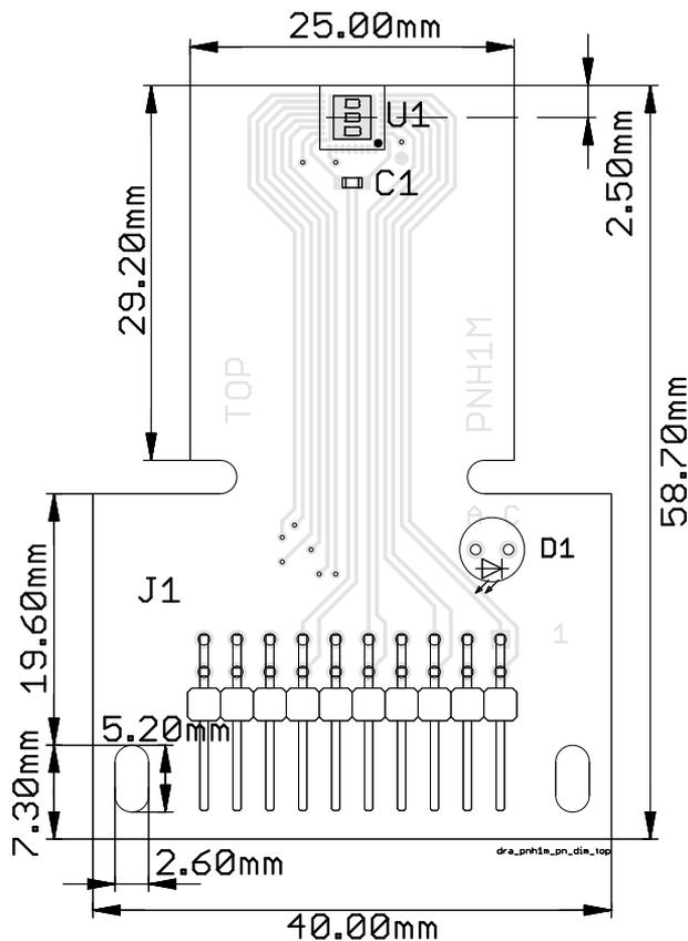
Figure 1: Sensor board PNH1M (top view)
