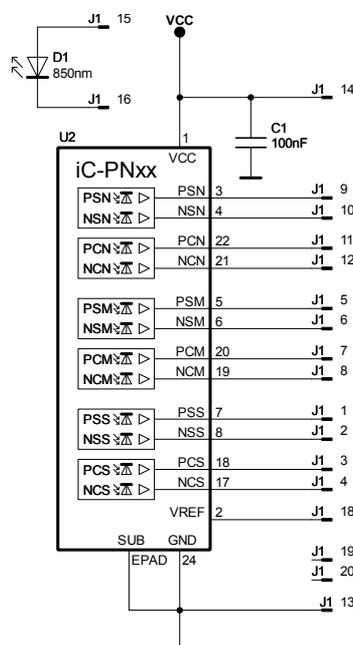
Figure 3: Circuit diagram
