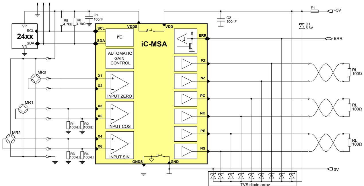
Figure 8: Example circuit for safety-related applications with iC-MSA.
