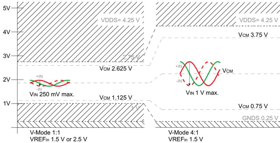
NB:  $V_{REFin}$  is referenced to GNDS.
