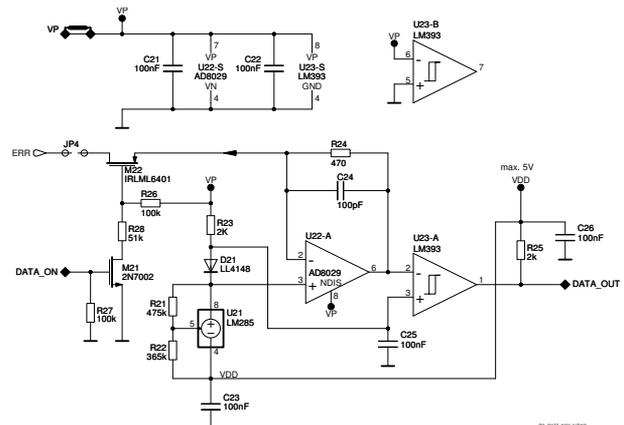
Figure 1: Example circuit for the decoding and conversion of the current-modulated signals to logic levels.
