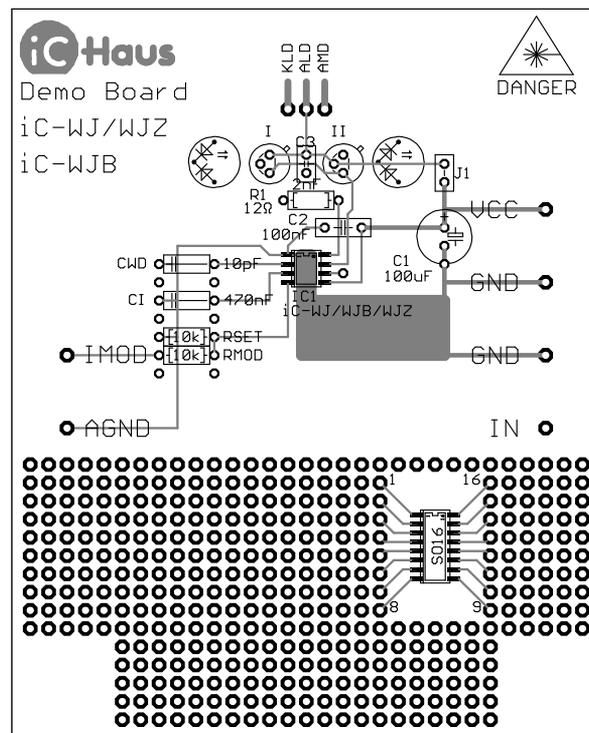
Figure 13: Demo Board (components side)
