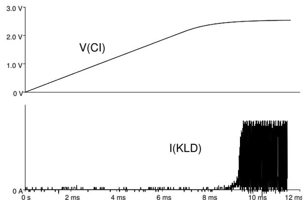
Figure 5: Turn-on behavior,  $f(IN) = 100 kHz (1:1)$ ,  $CI = 470 nF$ ,  $RSET = 10 k\Omega$
