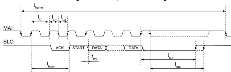
Figure 6: BiSS C protocol timing (ACQMODE  $\neq$  00)
