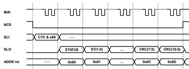
Figure 29: Cyclic readout
