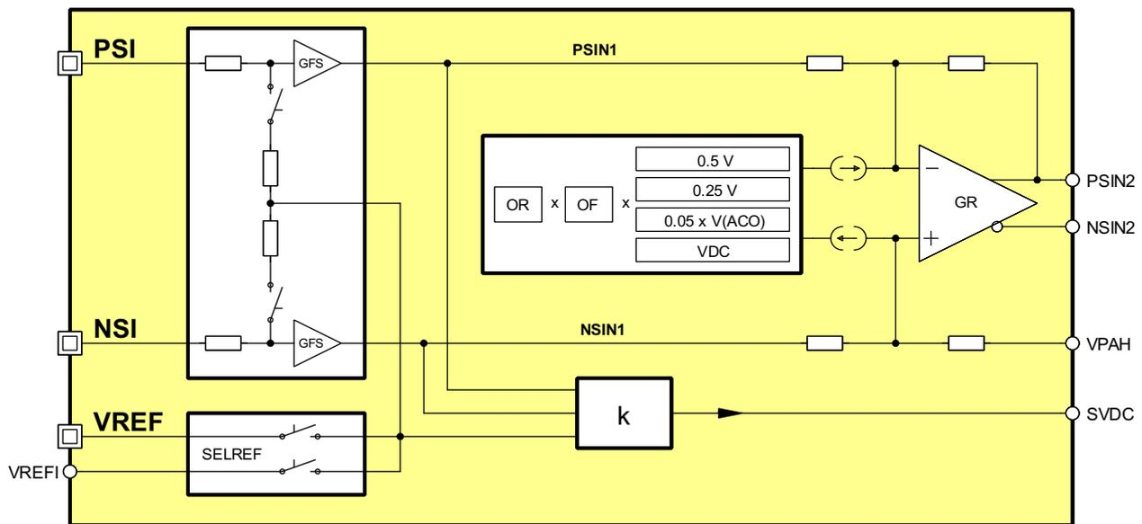
Figure 9: Signal-conditioning unit (sine channel)
