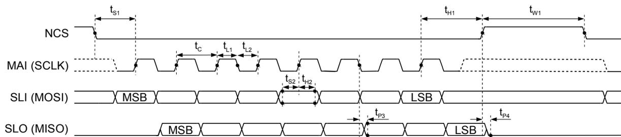
Figure 8: SPI protocol timing
