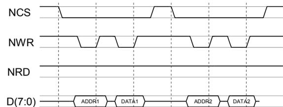
Figure 22: Write process
