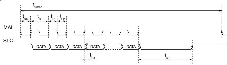
Figure 5: SSI protocol timing
