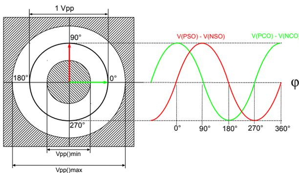
Figure 13: AC level monitoring: differential voltage thresholds according to Elec. Char. Nos. B01 and B02. For error messaging refer to diagnosis register, page 47.
