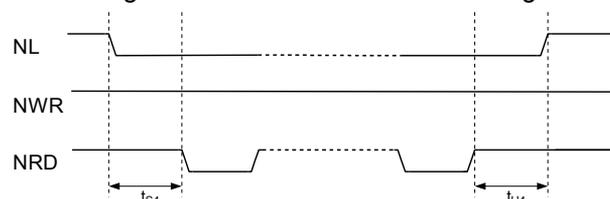
Figure 4: Parallel I/O interface timing for pin NL
