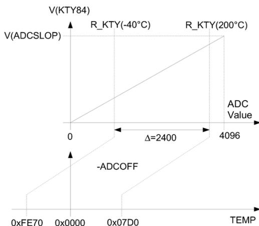
Figure 15: Calibrating the temperature sensor to the output format
