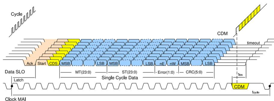
Figure 25: Example of line signals (BiSS C)
