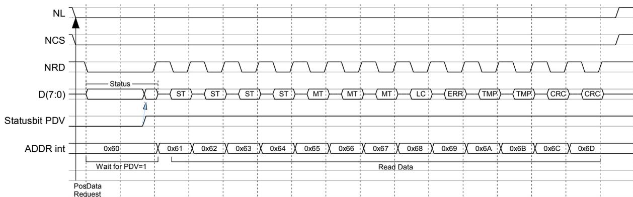
Figure 24: Position data output at request by pin NL
