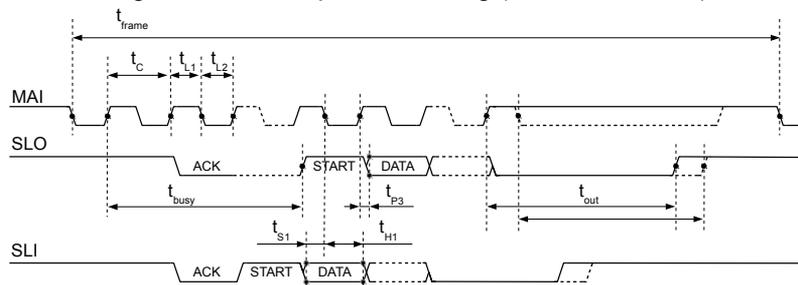
Figure 7: BiSS C protocol timing with triggered conversion (ACQMODE = 00) and chain operation
