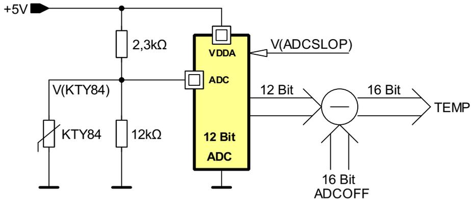
Figure 14: Schematic circuit diagram for the evaluation of KTY sensors.
