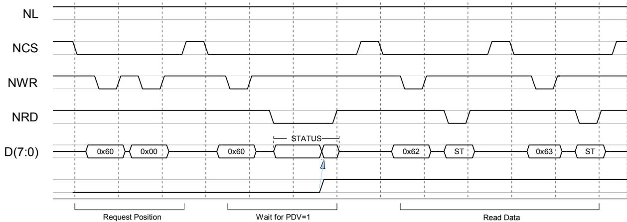
Figure 23: Position data output at request by command
