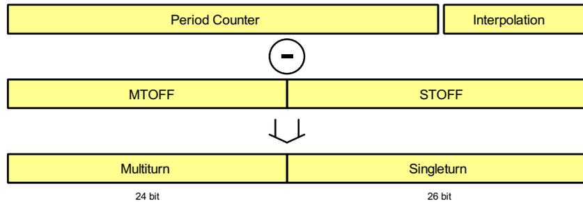
Figure 17: Position data generation with offset correction
