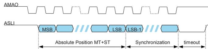
Figure 20: ADI data frame with SSI protocol
