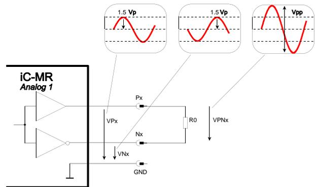
Figure 10: Measuring the differential signal amplitudes
