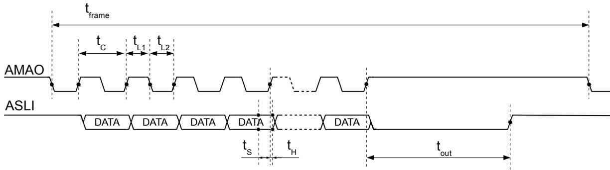
Figure 2: ADI timing with SSI protocol
