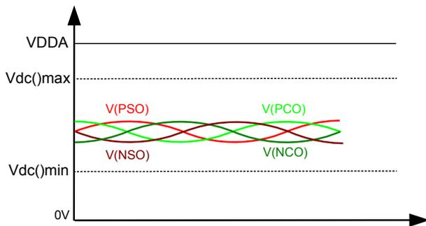
Figure 12: DC level monitoring: max. and min. voltage thresholds according to Elec. Char. Nos. B04 and B05. For error messaging refer to diagnosis register, page 47.
