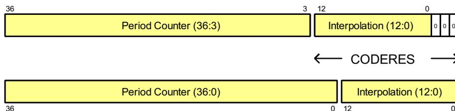
Figure 16: Adjusting the counter depth
