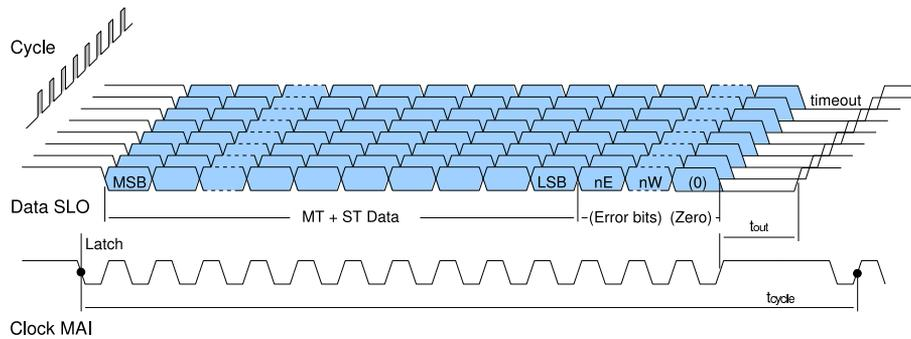
Figure 26: Example of line signals (SSI)
