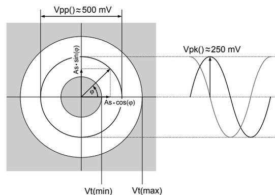
Figure 11: Control monitoring according to setpoint of square control (example: ACOC = 0x19; for Vt()min or Vt()max; see Elec. Char. Nos. 809 and 810).
