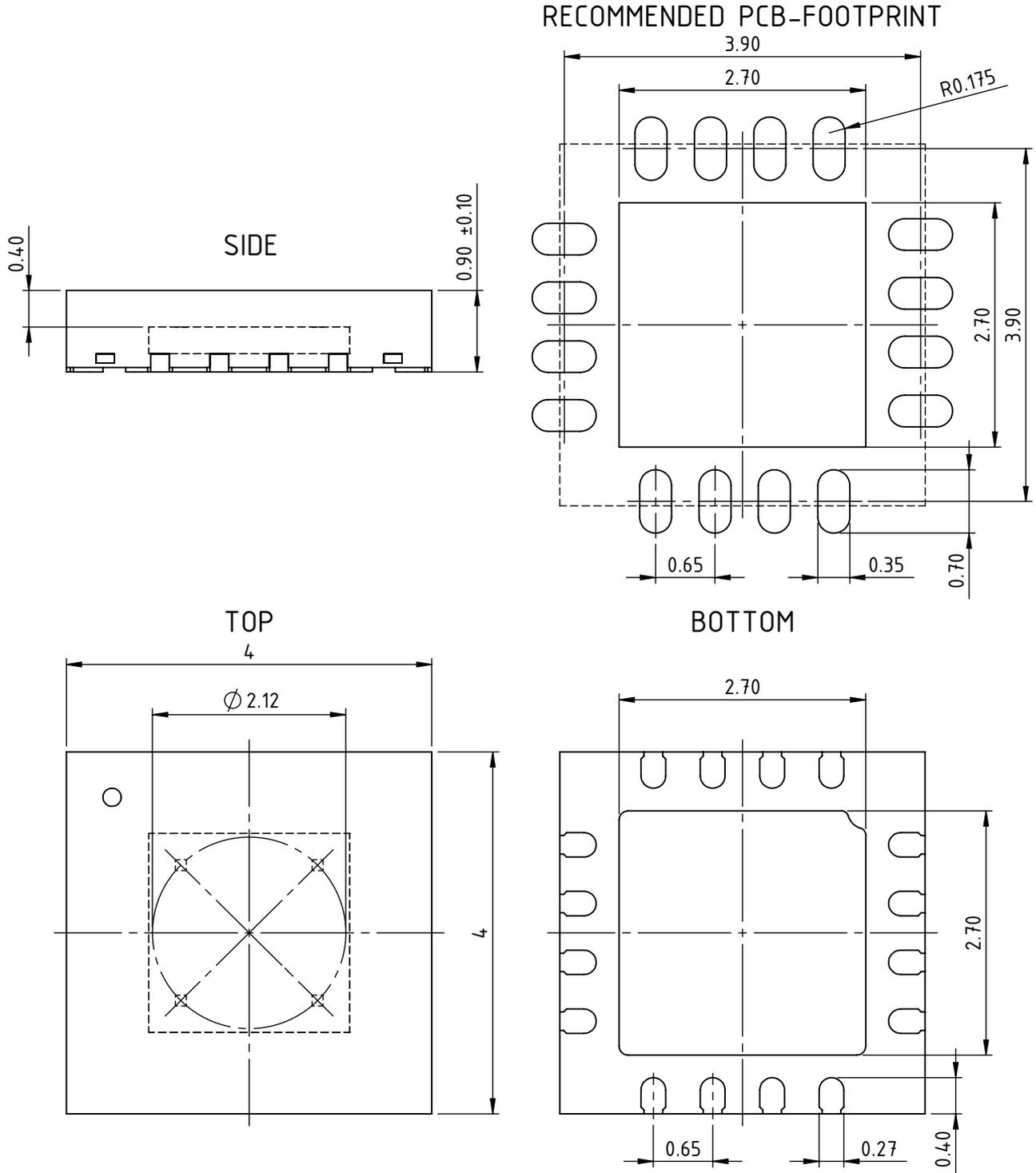
All dimensions given in mm. Tolerances of form and position according to JEDEC MO-220.
