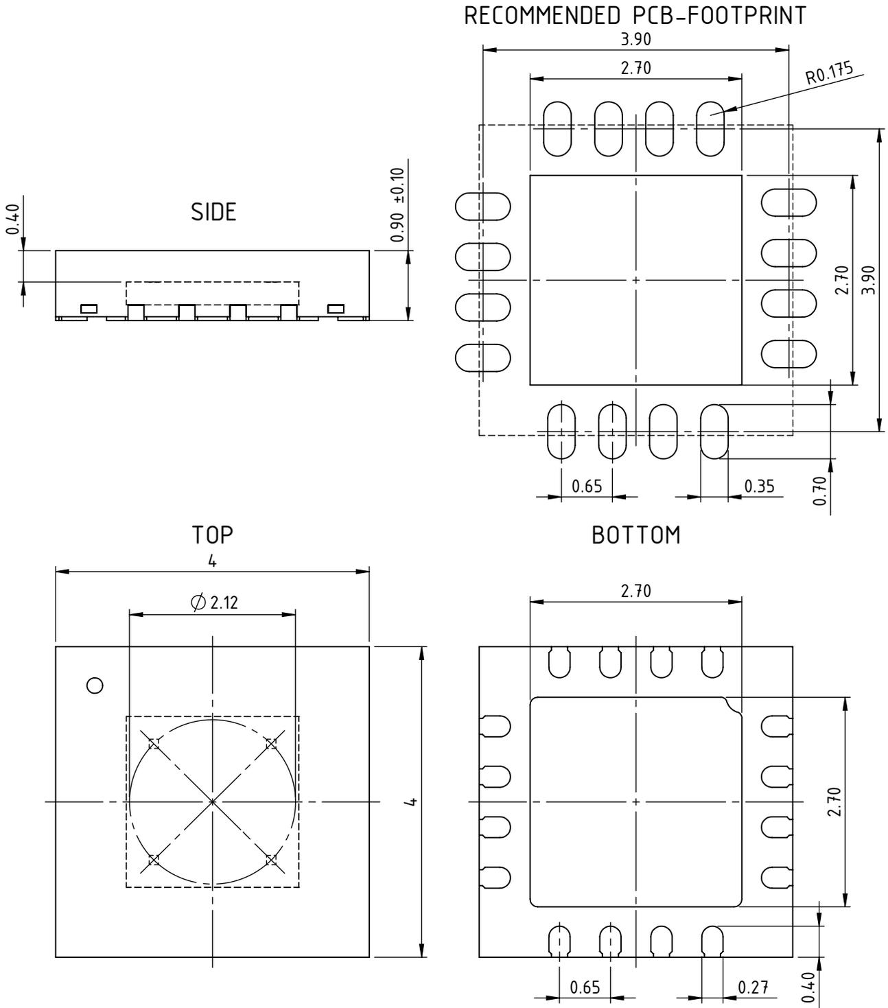
All dimensions given in mm. Tolerances of form and position according to JEDEC MO-220.
