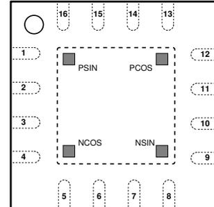
Figure 2: Position of the Hall sensors in the QFN package (top view)
