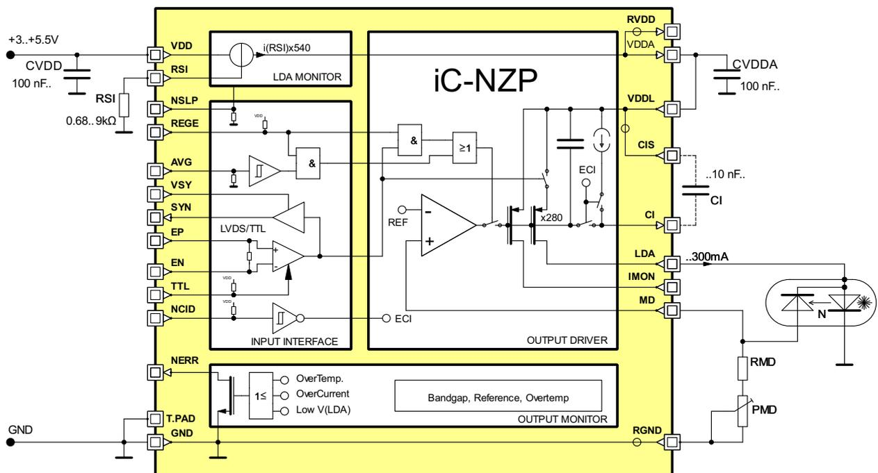
Figure 5: Circuit example for N-type laser diodes
