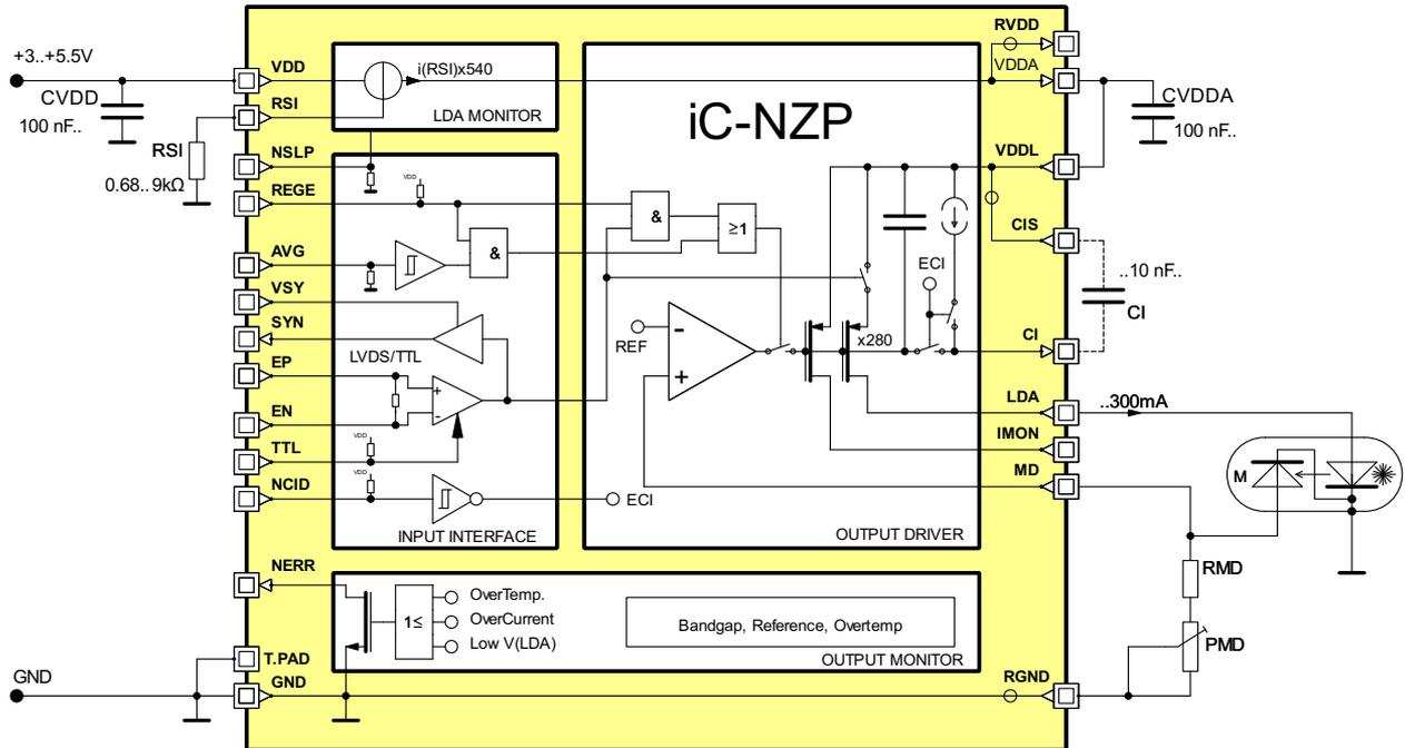
Figure 4: Circuit example for M-type laser diodes (case grounded)
