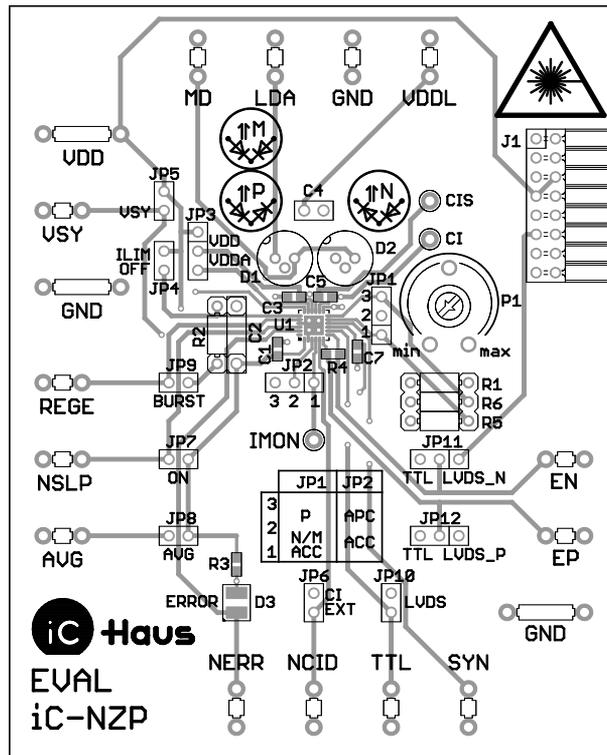
Figure 9: Evaluation board (component side)
