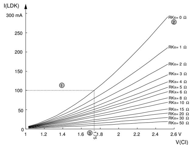
Figure 8: Diode current vs. V(CI) at T<sub>j</sub> = 27 °C
