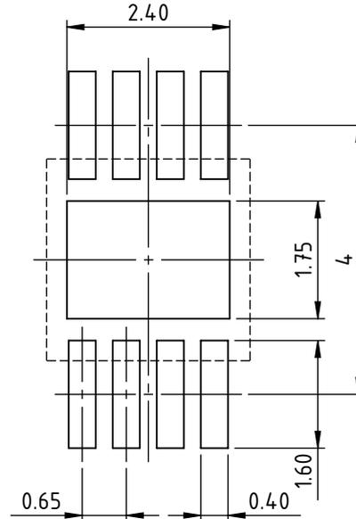
All dimensions given in mm. Tolerances of form and position according to JEDEC MO-187.
