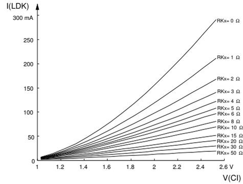
Figure 2: Diode current vs. V(CI) at T<sub>j</sub> = 27 °C
