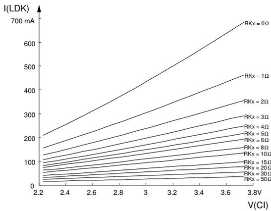
Figure 3: Diode current vs. V(CI) at T<sub>j</sub> = 27 °C
