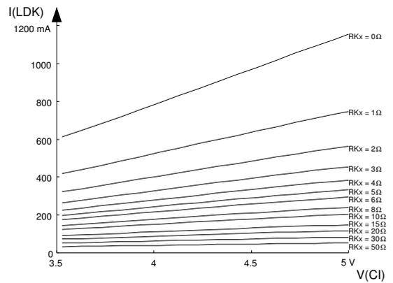
Figure 4: Diode current vs. V(CI) at T<sub>j</sub> = 27 °C
