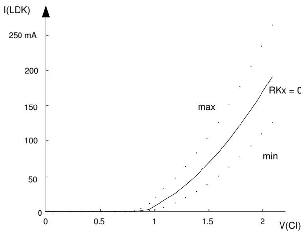
Figure 5: Diode current variation vs. V(CI) at V(LDK) = 3 V
