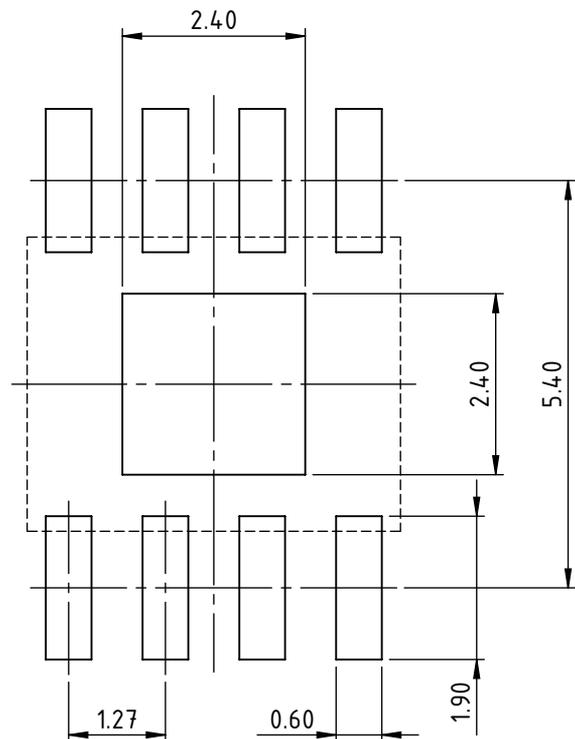
All dimensions given in mm. Tolerances of form and position according to JEDEC MS-012
