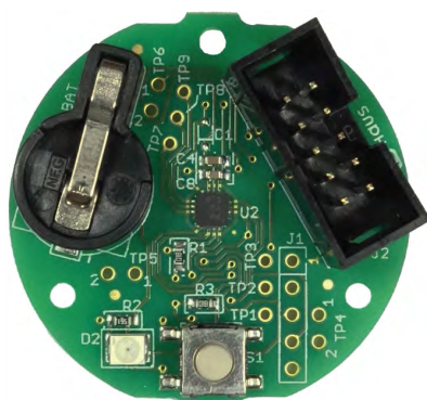
Figure 1: PV1M1 with iC-PV on top side.
